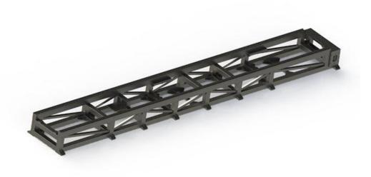
The crossbeam adopts a steel structure welding process, which is formed by precision mechanical processing after overall annealing, reducing weight and improving rigidity. This greatly improves the response speed of the machine tool.
